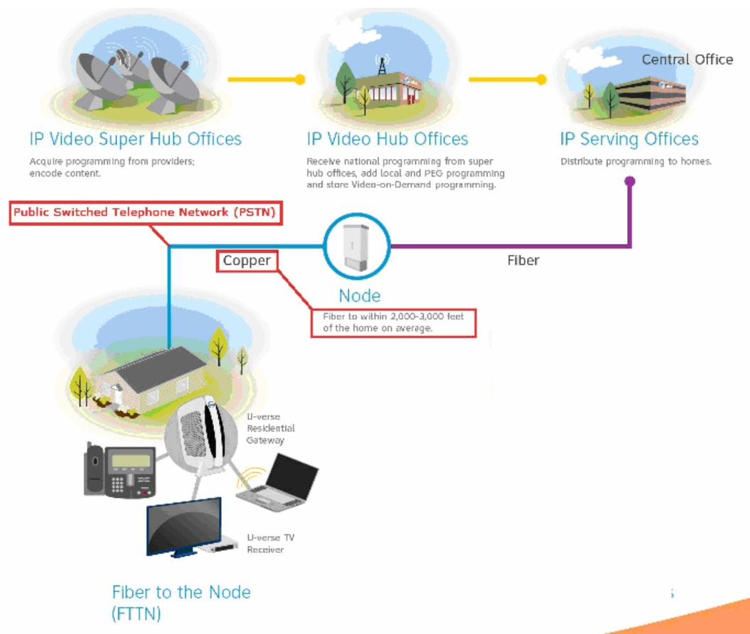
And in this diagram, AT&T didn't bother to properly label the graphic with the fact that the "copper" wire is the 10-50 year old PSTN wires, which we added in red.
